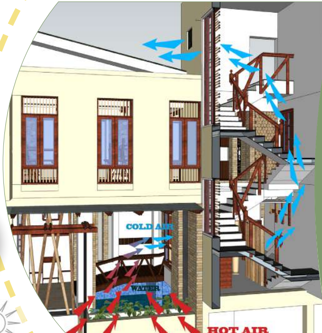
Sketch illustrating direct evaporative cooling on-site, highlighting the strategic placement of water bodies and the role of natural ventilation in enhancing thermal comfort
