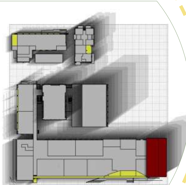
Diagram showing the shadows of the building to create self shading among building blocks to reduce heat gain
